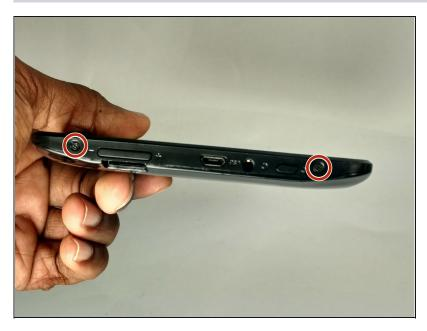
Use a Phillips 00 bit to remove two 3mm screws from the bottom of the tablet.
