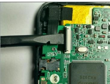
• Using the spudger to raise the zero insertion force (ZIF) connector to freely release the ribbon.
