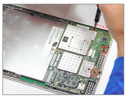
Remove the 2 – 3.5 mm screws from the motherboard assembly.
