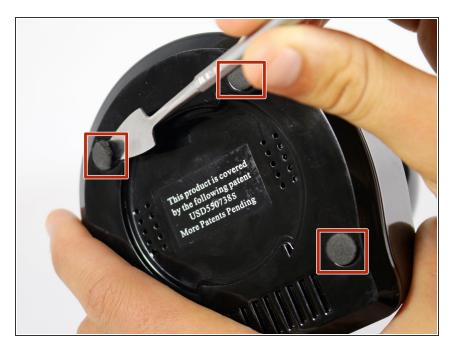
Remove the four bottom tabs in order to access the bottom screws.
