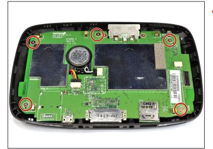
• Unscrew the five 4mm screws using the Phillips #0 screwdriver.
