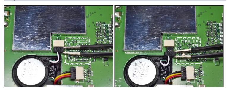
Unplug the connector shown near the center of the motherboard using the tweezers.
