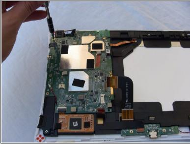
Remove the four 4mm Phillips screws with the PH#0 screwdriver.
