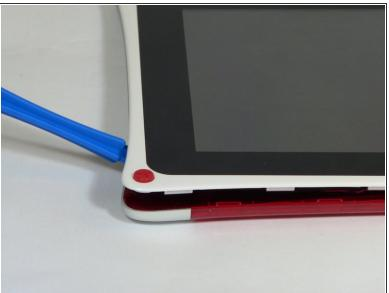
Use the plastic opening tool at the top left corner seam, then pry the corner apart.
