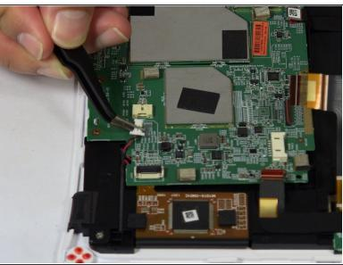
Disconnect the Right speaker by grabbing the wire head by its sides and pulling it back from the connector.
