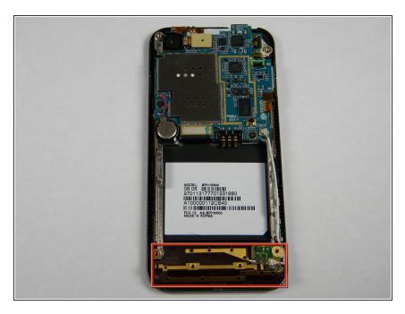
With the screws removed, locate the antenna.
