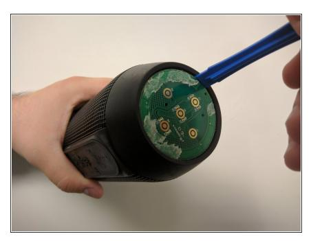
Use your plastic opening tool to pry the button board loose by lifting the edges.
