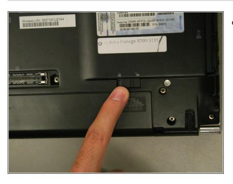
Locate the battery lock button and push it towards the unlock position.
