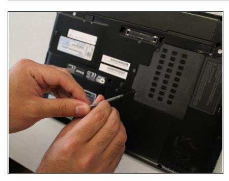
Using a Phillips #00 Screwdriver unscrew the 2 40mm screws that are located on the plate covering the RAM.
