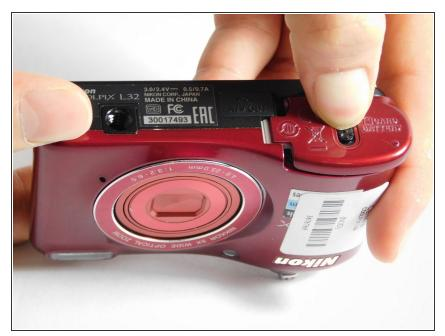
Slide the lock button on the battery compartment away from you while sliding the battery compartment door to the right to open the battery compartment door.
