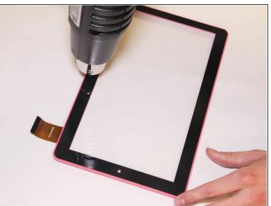
With a heat gun, heat along the border of the screen and case to weaken the glue.
