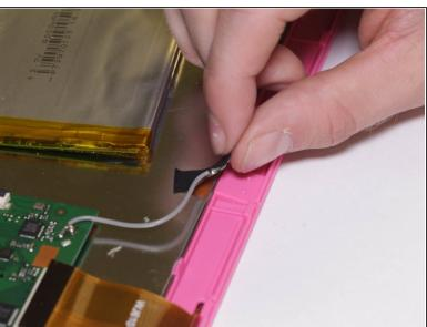
Carefully peel off these two pieces of tape to remove the antenna.
