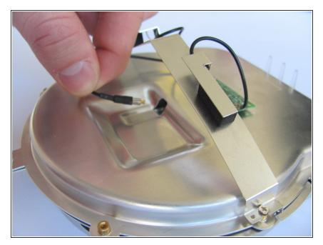
Unplug the black connector on the top of the metal casing by gently pulling horizontally.
