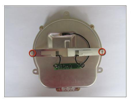
Remove the two 4mm phillips screws to remove antenna.
