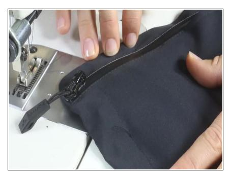
The last step is to re-sew the hem seam. If any sewing holes are still visible in the jacket, you can close them using the steam setting on an iron. Be sure that the iron does not touch the jacket!
