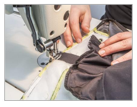
Position the pocket attachment correctly and sew it on to the closure edge.
