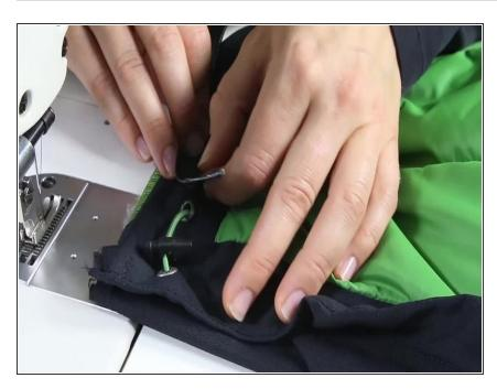
Sew the remaining zip half (without flap) onto the other side of the open jacket.
