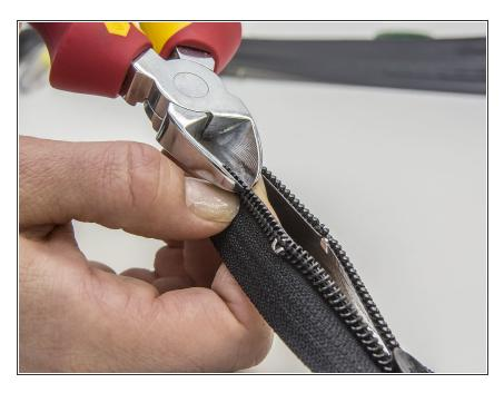
Use the wire cutters to pry off the zip teeth after the stopper.
