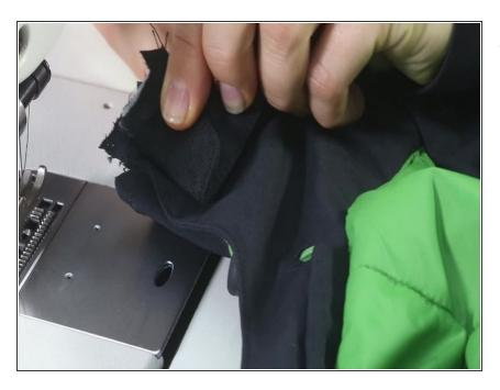
Sew the front flap with the zip attached onto the jacket lining.
