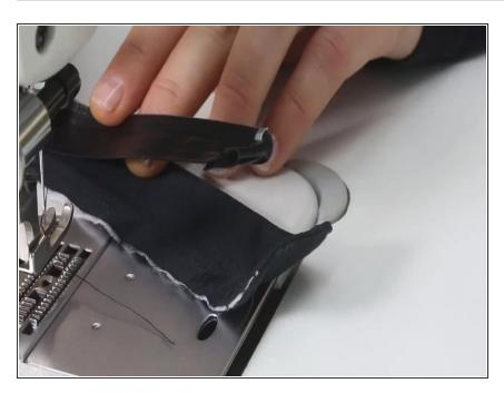
Sew the zip onto the front flap using the zip foot.
