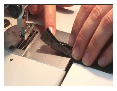
Fold over the seam allowance of the zip and sew it down with the sewing machine.
