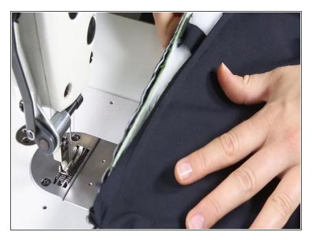
Then sew the second side of the zip on. Move the slider as you sew to keep it out of the way.
