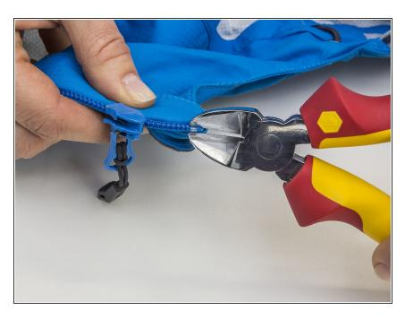
Remove the zip stop at the end of the zip by prying it open with a wire cutter and pulling it away.
