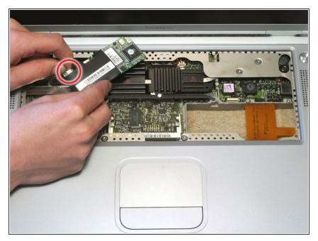
• Disconnect the connector cable from the modem.
