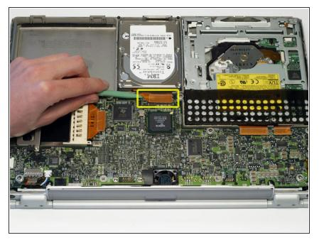
Disconnect the hard drive ribbon from the logic board using a spudger or the tip of your finger.
