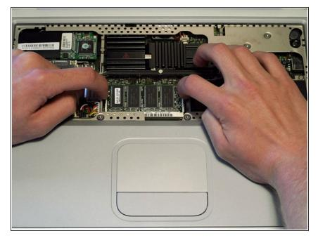
Release the tabs on each side of the RAM chip at the same time. These tabs lock the chip in place and
