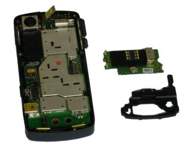
Use a plastic opening tool to pry the two ribbon cable connectors, unclipping them from their sockets on the motherboard.
