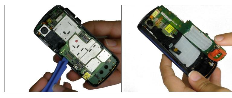
Use a plastic opening tool to gently pry the motherboard up until you can tilt it with your fingers.
