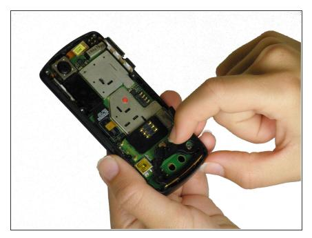
Lift the black rubber loudspeaker housing up and out of the plastic casing.
