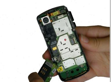
• Use a plastic opening tool to gently lift up the SIM card reader, located above the rubber antenna casing. You should hear a click as it releases.
