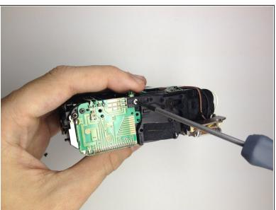
Use the Phillips #00 Precision Screwdriver to remove the screws.
