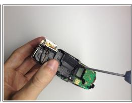
Remove the 3 screws using the Phillips #00 Precision Screwdriver.
