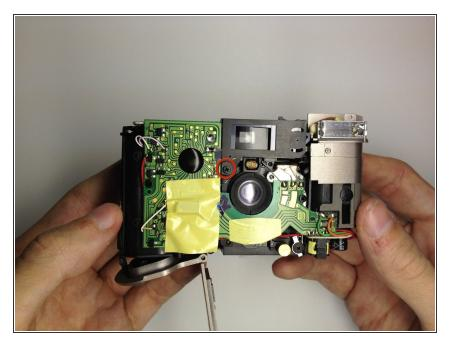
Locate the screw on the front of the camera that holds the view finder assembly.
