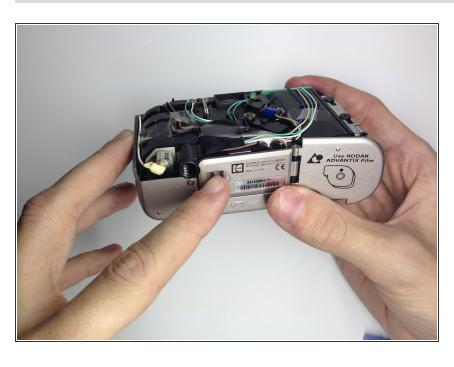
Open the battery door by pushing the lever towards the arrow indicated.
