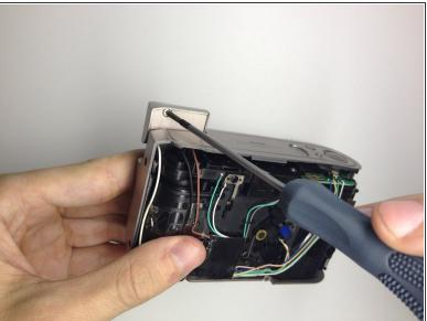
• Remove the screw located under the flash module using the Phillips #00 Precision Screwdriver.
