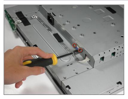
Using a 5 mm nut driver, unscrew the VGA port's mounting screws from the metal casing.
