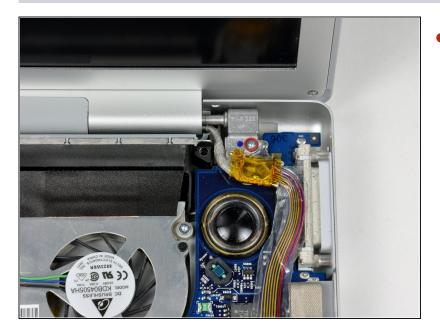
• Remove the silver 9.5 mm T6 Torx screw securing the ground loop in the display data cable to the casing.
