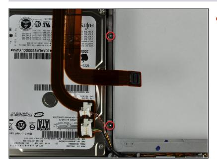
Remove the two silver T6 Torx screws securing the hard drive retaining bracket to the lower case.
