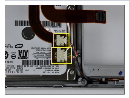
Disconnect the IR and sleep light cables from their connectors above the hard drive, removing tape as necessary.
