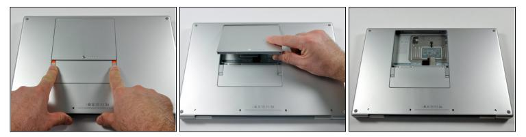
• Use your fingers to push both battery release tabs away from the battery, and lift the battery out of the computer.
