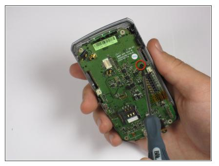
• Remove the 3.4 mm black screw with the Phillips #000 screwdriver.
