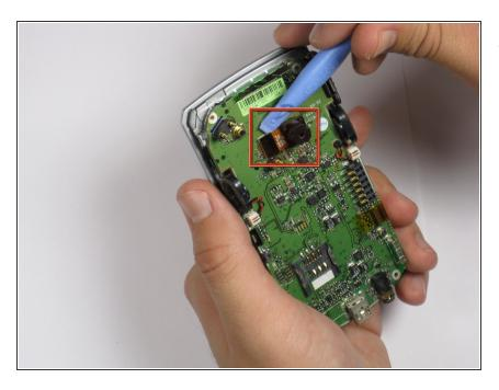
• Locate the camera and pry off with the plastic opening tool or spudger.
