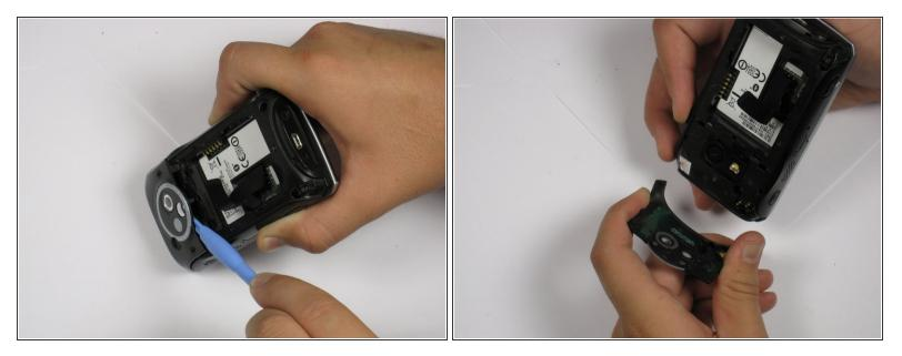
• Use a plastic opening tool to remove the camera cover.
