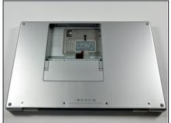
• Use your fingers to push both battery release tabs away from the battery, and lift the battery out of the computer.
