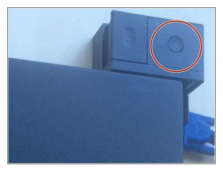
Turn off the screen and press the ON button shown, the docking station
