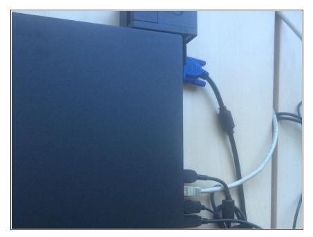
Connect the necessary power, monitor (VGA), etc. cables to the docking station
