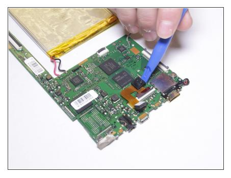
• Locate the rear camera and use a prying tool to gently lift the rear camera off of the motherboard.
