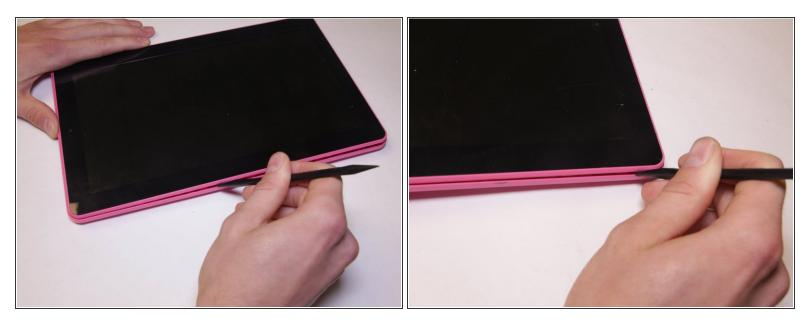
• Use a spudger to pry the back cover. Start from one edge of the back cover and slide across until the cover is lifted from the tablet body. Repeat for all edges.
