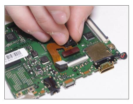
Detach the camera ribbon wire by lifting the tab and pulling the wire. This will leave you with the camera assembly.
