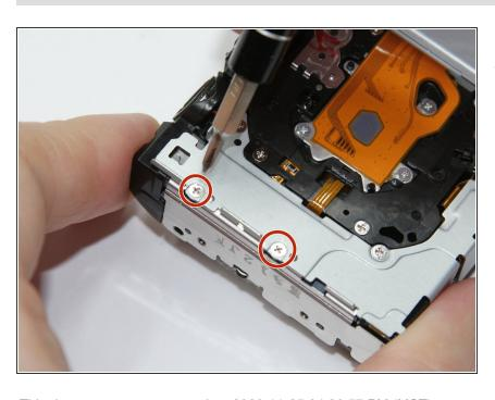
Remove the two screws (2 mm
