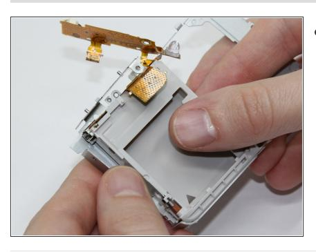
Lift out the battery tray. The button ribbon assembly will come with it.
