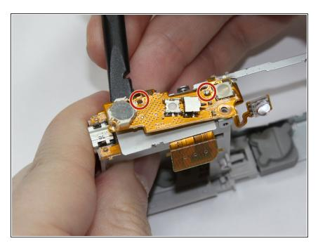
Use the spudger to lift the shutter button ribbon up out of the alignment tabs.
