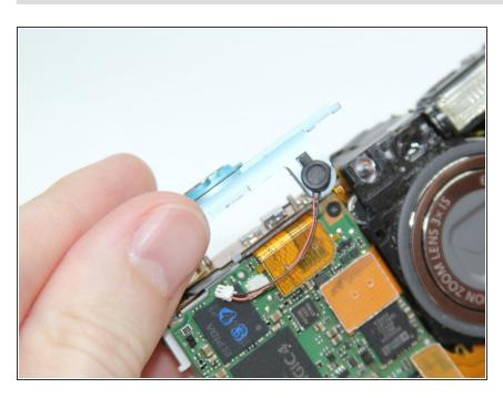
Lift off the mechanical shutter button assembly.
