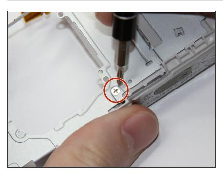
On the backside of the camera, remove the screw located at the bottom center of the metal frame beneath the lens assembly. (2.5mm Phillips 00)
