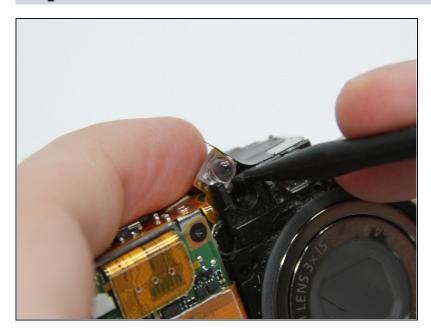
Use the spudger to gently lift out the LED at the top of the lens assembly.
