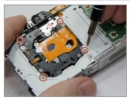
Remove the 4 corner screws on the back of the camera in silver metal frame surrounding the back of the lens assembly (2.5 mm Phillips 00).
