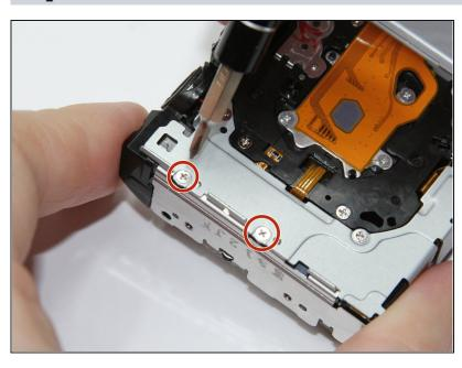
Remove the two screws (2 mm Phillips 00) along the back edge of the camera frame directly behind the flash assembly.
