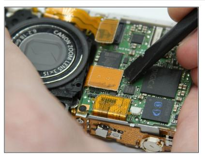
Use the spudger to gently pry up both sides of the flat-topped connector, then lift the cable directly up out of its socket.
