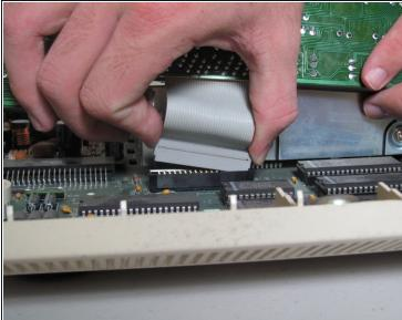
• Tilt the keyboard up while detaching the ribbon connection by pulling it straight up. You may have to wiggle the connector sideways to loosen it.
