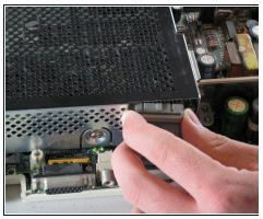
Carefully detach ribbon connector from floppy disk drive by pulling it out horizontally.
