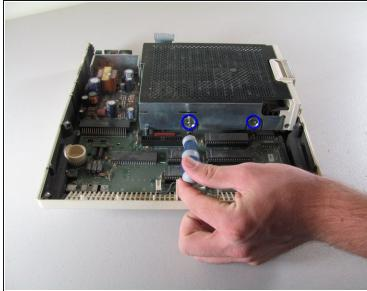
• Unscrew the four 8.5 mm screws that attach the floppy drive cage. Two screws are located on the front and back of the cage.
