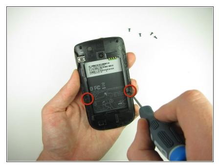
Remove the two 4.3mm Phillips #00 screws that secure the back panel to the rest of the phone.
