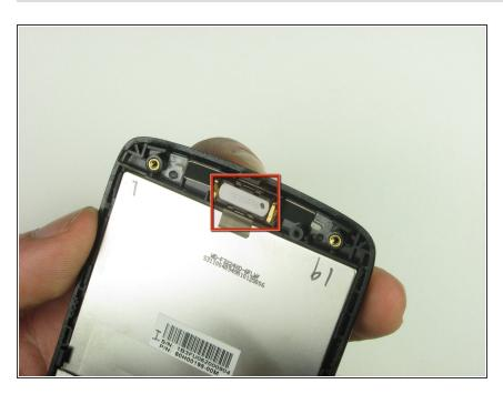
Locate the internal speaker at the top center of the phone.
