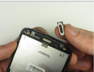
• Using the plastic opening tool, carefully pry out the internal speaker.
