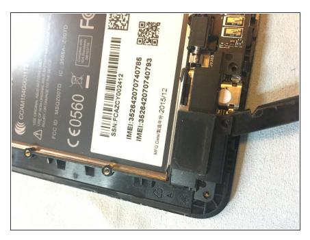
Use a spudger to pop off the loudspeaker. It is held to the case by a little adhesive.
