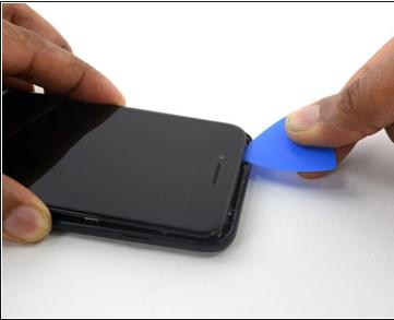
Slide an opening pick along the top edge of the iPhone, between the rear case and front panel, to break up the remaining adhesive holding the screen in place.
