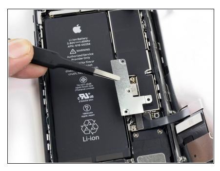
Remove the lower connector bracket.
