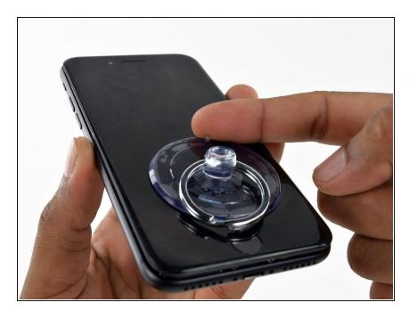
Pull up on the small nub on the suction cup to remove it from the front panel.
