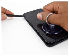
• Slide the spudger up the left side of the iPhone, starting at the lower edge and moving towards the volume control buttons and silent switch.
