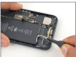
• Use a pair of <u>tweezers</u> with blunt tips to peel back one of the adhesive strips on the lower edge of the battery.
