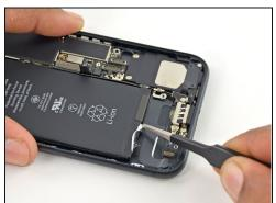
• Use a pair of tweezers with blunt tips to peel back one of the adhesive strips on the lower edge of the battery.
