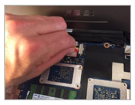
Grab wires in middle and pull and wiggle gently to pull out wires from connection.
