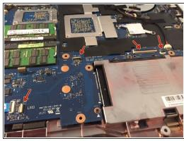
Slowly lift up keyboard to see the 4 ribbon cables and carefully pry up tabs where cables are connected.
