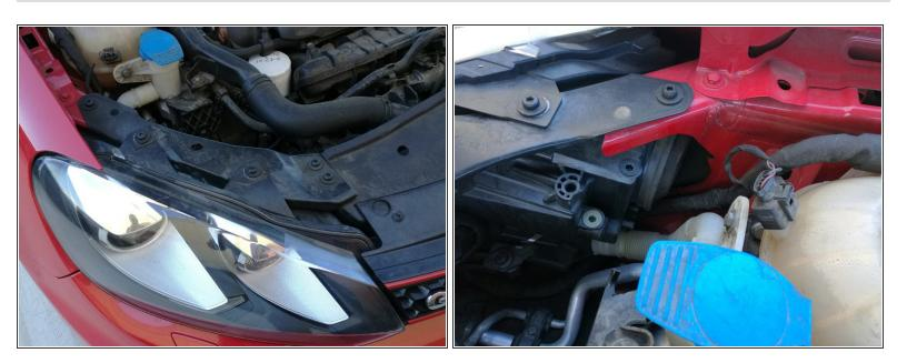
Open the hood and then locate the back of the headlights.
