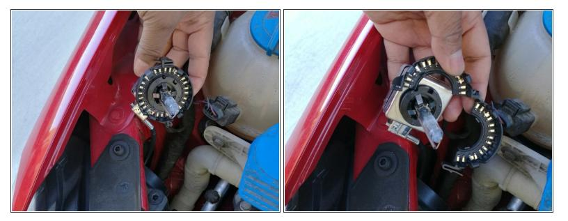
• For a lot of D1S and D3S, there's a bulb retainer, which you will need to remove.
