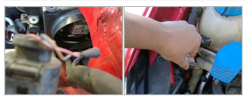
Once you can see the OEM headlight bulb, twist and unlock to take it out.
