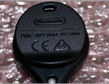
one phillips PH1 screw located on the back to remove the battery cover
