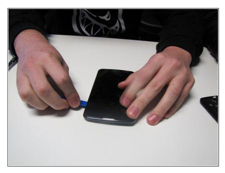
Unscrew every screw of the bottom of the phone and use guitar picks to remove the plastic frame of the phone
