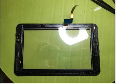
Remove any remaining adhesive and piece of glass to allow adhesive and glass panel replacement.
