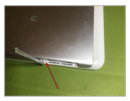
Open the SD slot and remove the screw hidden under the sticker.
