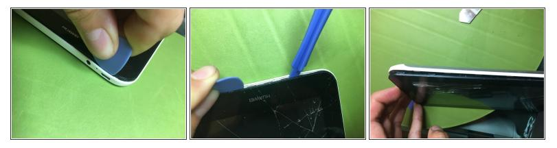
Use an opening pick to disengage the clips securing the back cover.
