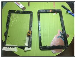
Apply heat on the panel edges. Use an opening pick to separate the glass panel from the plastic frame.
