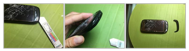
With a thin tool insert it in the cover at the bottom and pry up to release it
