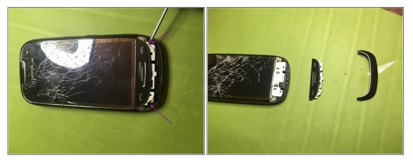
Pry up the two points indicated by the arrows to release the keyboard
