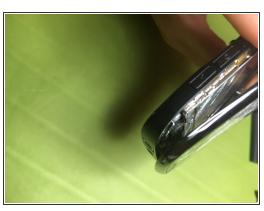
Gently lift the front glass and slide it slightly in the direction of the arrow so you can free it
