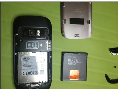
Remove battery and battery cover
