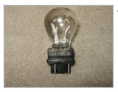
Replace the burned out bulb with a new type 3057 dual filament bulb
