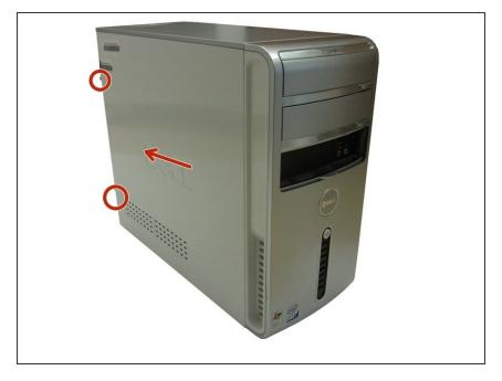
Remove the side panel, and and and screws that may be holding it in place.
