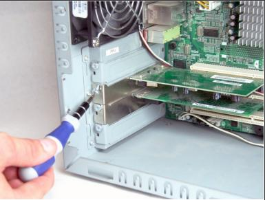
Remove the Torx T15 screwdriver holding the PCI card in place.
