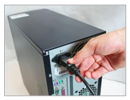
Turn off your computer and remove the power cable by pulling it straight out of its socket.
