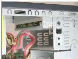
Remove the IDE data cable and the power cable from the optical drive by pulling away from the drive.
