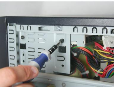
Remove the other 2 Torx T15 screws holding the other side of the drive in place.
