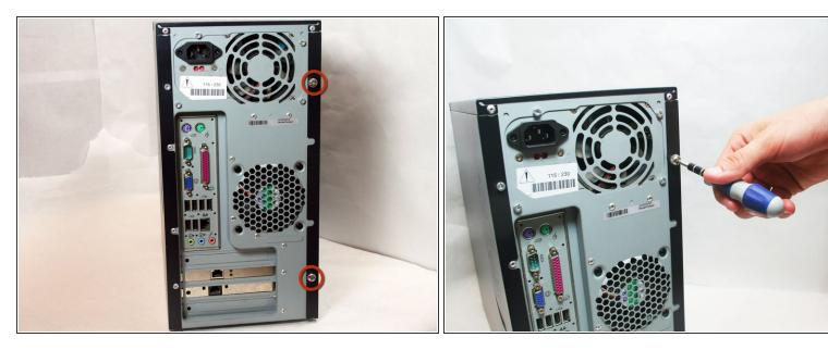
Remove the two Phillips #2 screws that secure the case door to the device.
