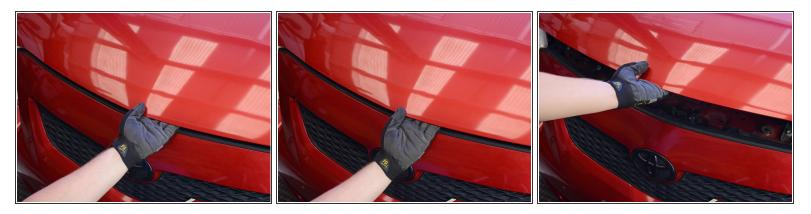
• Raise the hood by simultaneously lifting and pressing up on the hood latch release (usually located beneath the front edge of the hood, near the center or center-right).
