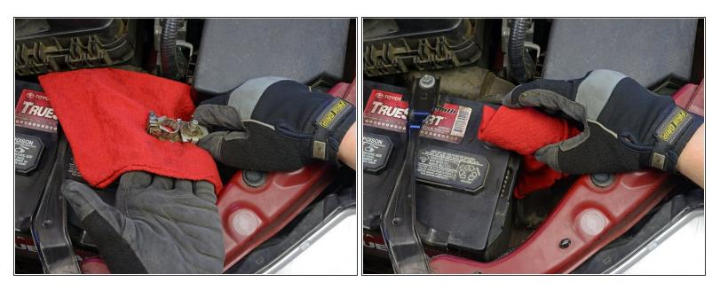
Prevent the cable from making accidental contact with the terminal by pushing it aside and/or wrapping the cable clamp with a dry rag.
