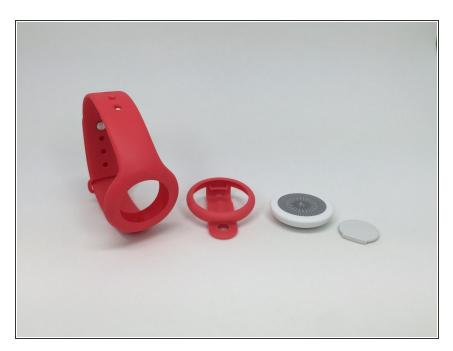
From left to right: silicone wristband, clip, tracker and plastic coin to open the casing
