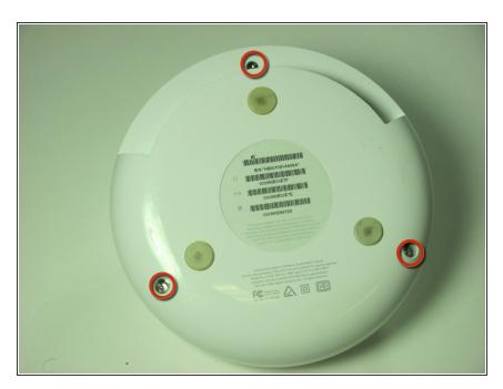
Remove the three 5mm T7 Torx screws from the back panel.
