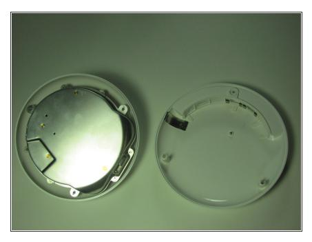
Separate the bottom and top casings.
