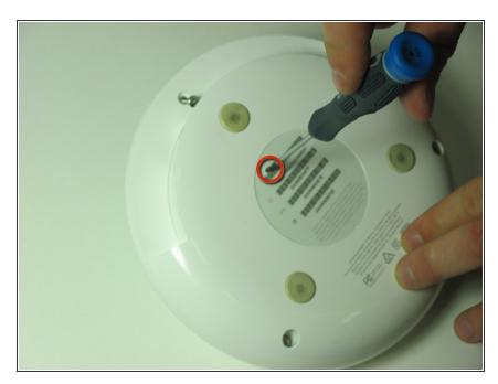
Remove one 5mm phillips screw located under the identification sticker. You will need to remove the sticker or make a hole to get to the screw.
