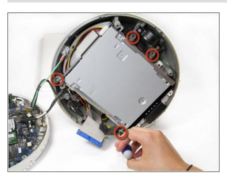
Using a Torx # 10 screw driver, remove the four 19.12mm screws that mount the optical drive.
