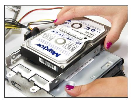
Slide the hard drive out of the assembly.
