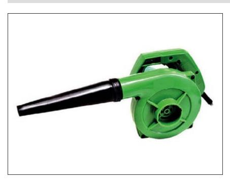
Blow air to the air conditioner with air blower but make sure that the air pressure does not get to the air reflectors of the unit.
