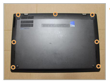
Loosen the seven cover screws.
