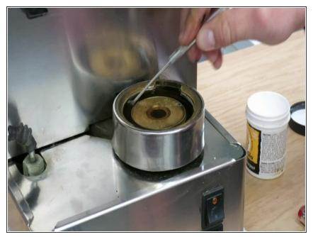
• Use a small flathead to clean the bottom surface of the grouphead.
