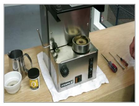
• Pry the gasket up with the sharp tip of the awl.
