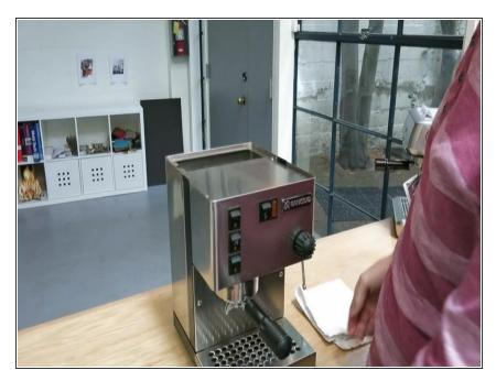
• Remove drip tray. Flip the machine upside down.
