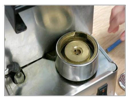
• Insert the diffuser with the water channels facing down.
