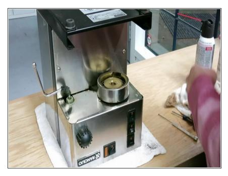
• Use the compressed air can to clean any excess water or coffee.
