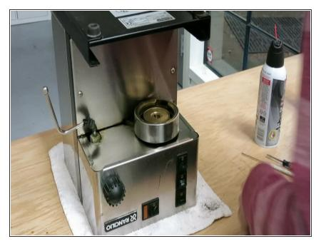
• Last but not least, use the pick on the top and bottom rails to remove last bits of coffee debris.
