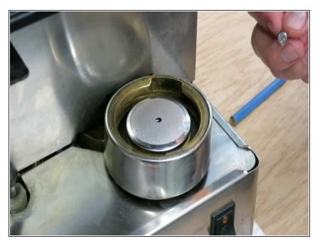
• Use an 8mm socket wrench to tighten the screw.
