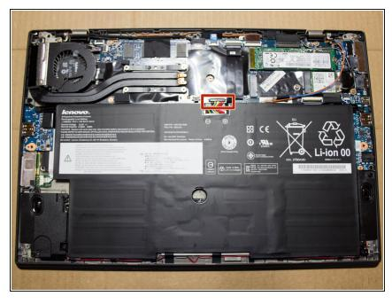
⚠ Disconnect the battery connector from the main board by pulling the connector towards the battery.
