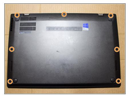
Use phillips #2 screwdriver to loosen seven cover screws.
