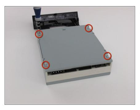
Unscrew the four 8.5 mm screws on the bottom chassis using a Philips #2 screwdriver.
