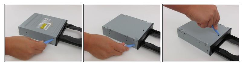
• Use an opening device to push in the black tabs on the left, right and bottom of the outer chassis to unhook the faceplate.
